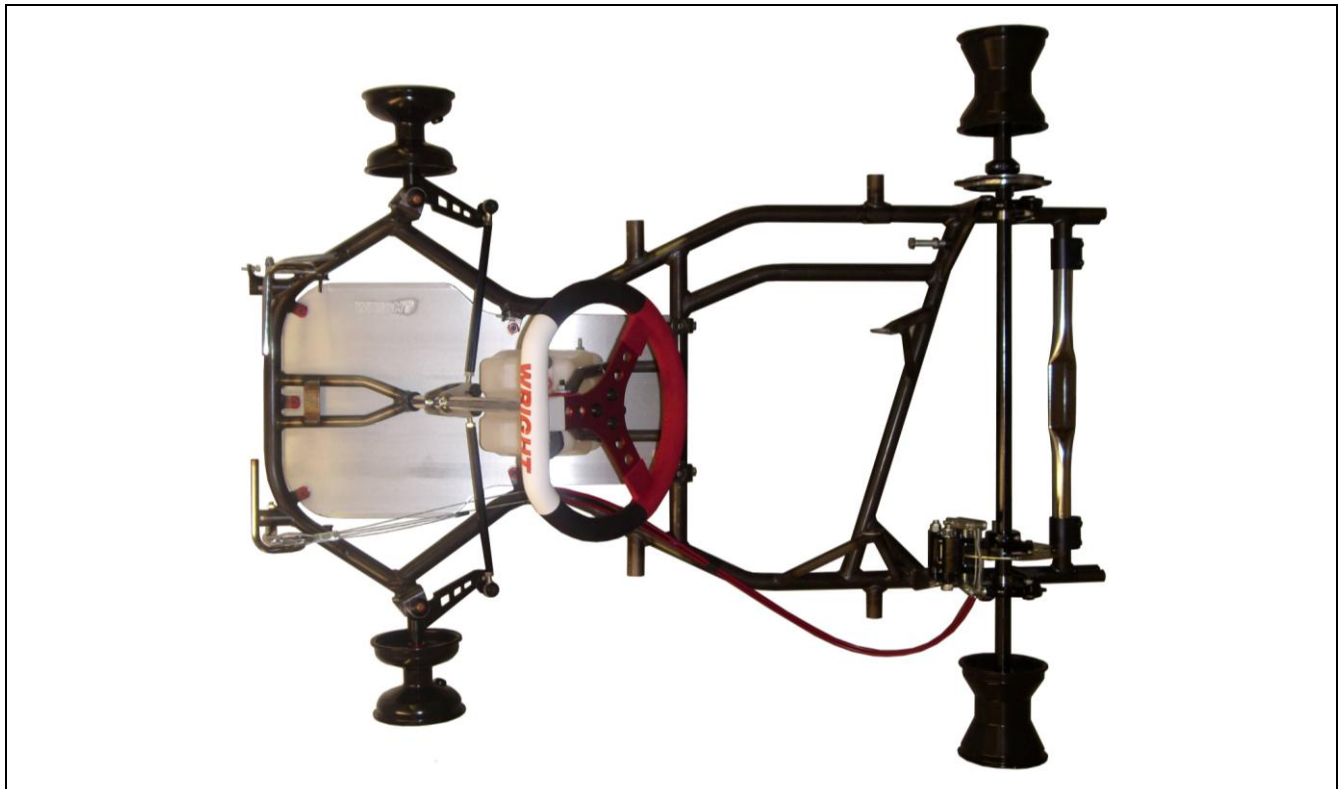
Photograph of complete chassis less seat and bumpers
