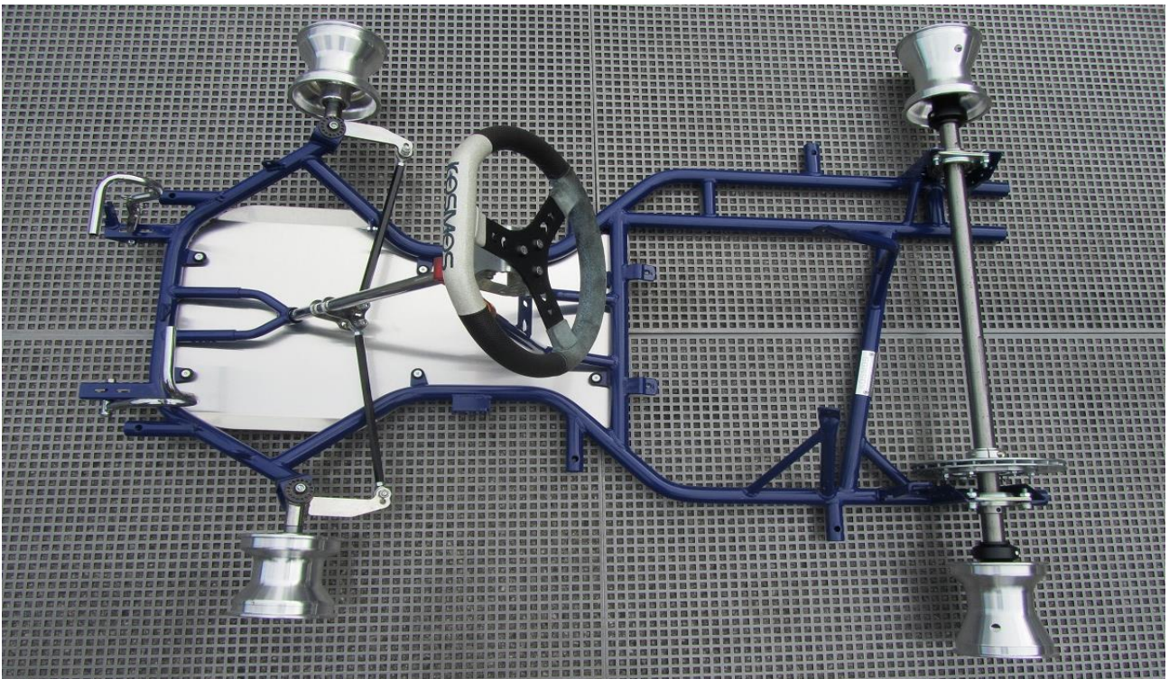
Photograph of the chassis less seat, brakes, tyres, bumpers and bodywork
