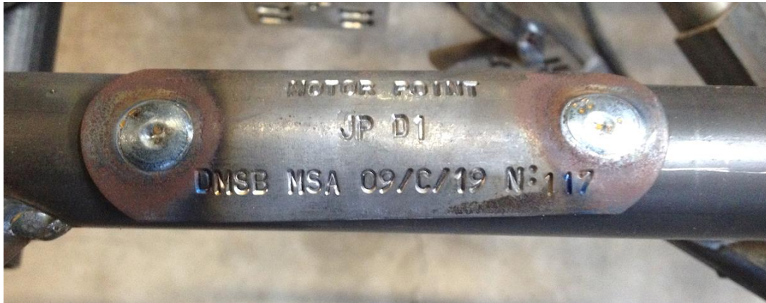
Photograph of Homologation Number marking
