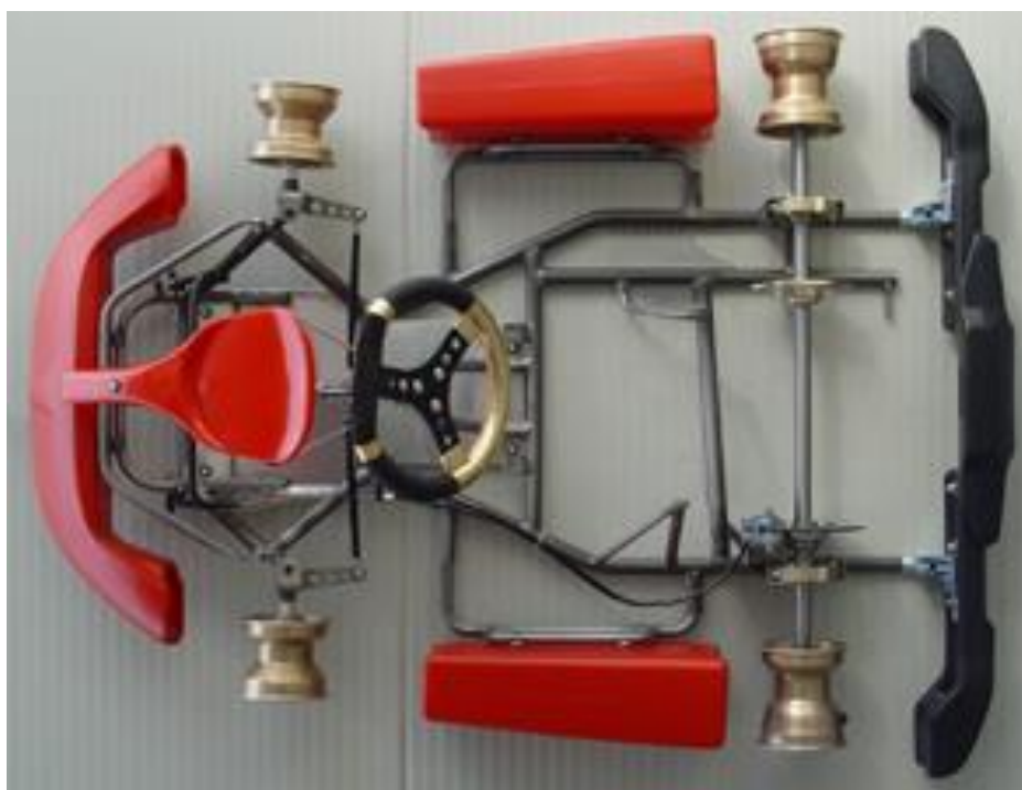
Photograph of complete kart less seat & tyres
