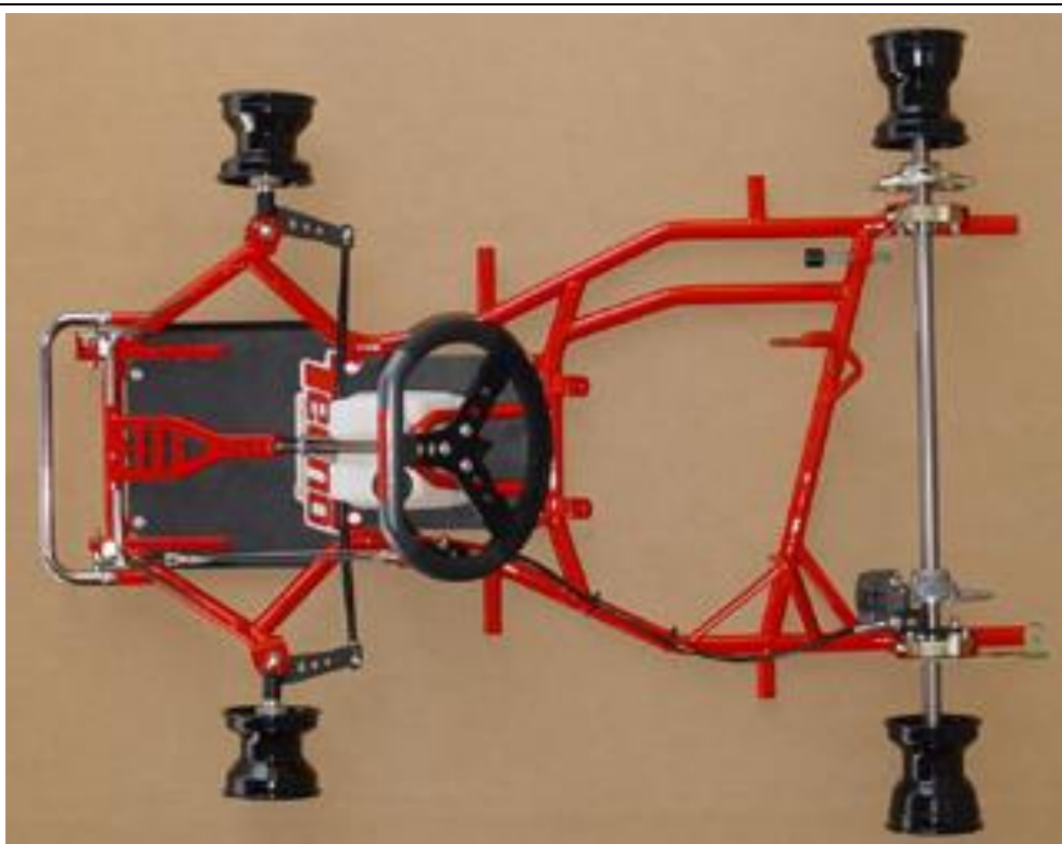
Photograph of complete chassis less seat and bumpers
