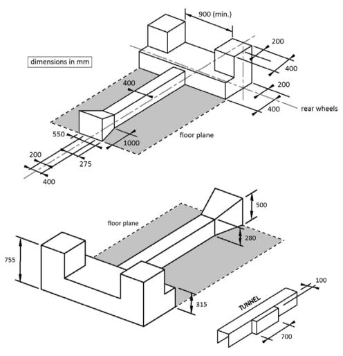
If any modifications have been made to the front or rear bulkheads, transmission tunnel or floor pan all the dimensions marked A-Q must be completed in the table in section 1.2(a).
