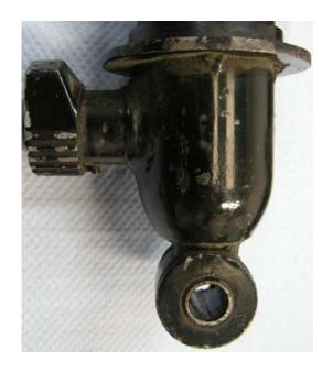
Twin tube dampers may incorporate valves in the base, the top gland and the piston, It is relatively simple to manufacture a damper with a user adjustable bump valve in the base and this technology was certainly in use on cars from the early 1950s.
