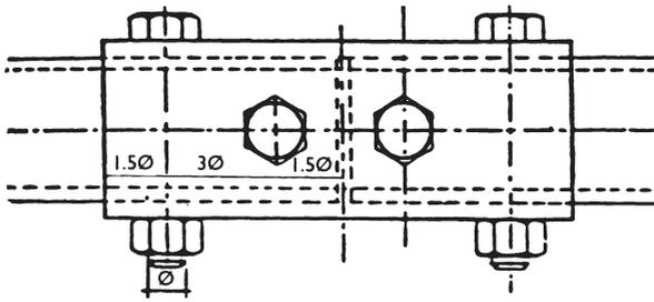
$\varnothing = 14\text{mm}$  (tube  $\geq 40\text{mm} < 50\text{mm}$  diam. ext.)
