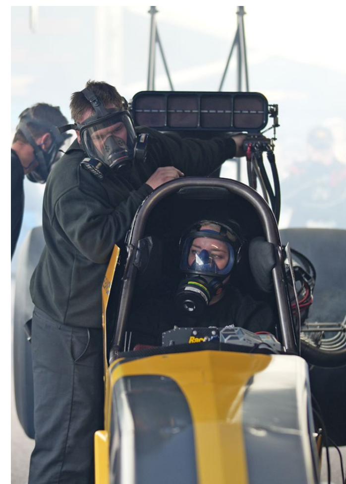
Nitromethane fumes are like teargas. Gas masks are often worn when Top Fuel engines warm up in the pits
