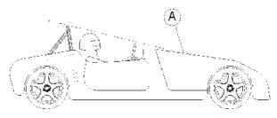
A' is the substantial structure forward of the driver such as to act as the front rollbar. No part of the driver's helmet is to pass through a line struck from the top of the rollbar to this structure.
