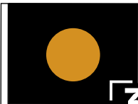
Black, Orange disc Mechanical failure
