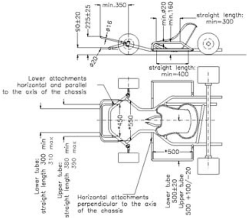
*Lower Tube  $\varnothing$  20mm
