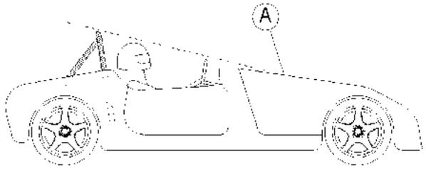
'A' is the substantial structure forward of the driver such as to act as the front rollbar. No part of the driver's helmet is to pass through a line struck from the top of the rollbar to this structure.
