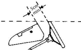
Bubbleshield profile showing horizontal line it must not cross and the minimum 5cm gap between the shield and steering wheel.
