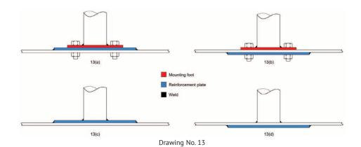
Rivetted or welded nuts
