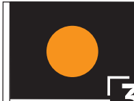
Black, Orange disc Mechanical failure
